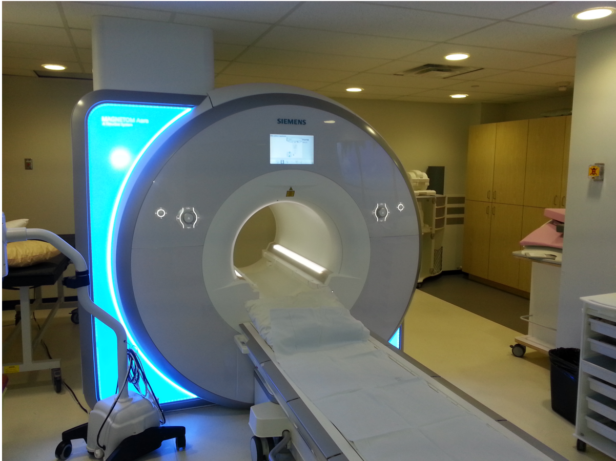
Figure 1.3: Seimens Avanto 1.5 Tesla MR scanner. A spine coil is located under the blanket.
